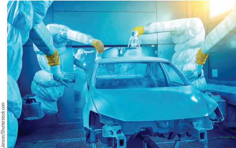
Figure 2-12: A robotic arm painting a car
